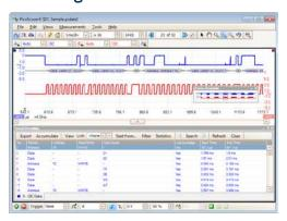
The PicoScope 2000 Series includes serial decoding capability as standard. Protocols currently included are  $I^2C$ , SPI, RS232/UART and CAN bus. Expect this list to grow as we release free software updates.
