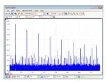
With the click of a button, you can display a spectrum plot of selected channels. The spectrum analyzer allows signals up to the full scope bandwidth to be viewed in the frequency domain. A full range of settings gives you control over the number of spectrum bands, window types and display modes: instantaneous, average, or peak-hold.
