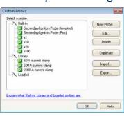
The custom probes feature allows you to correct for gain, attenuation, offsets and nonlinearities in special probes, or to convert to different units of measurement (such as current, power or temperature). You can save definitions to disk for later use. Definitions for standard Pico-supplied oscilloscope probes and current clamps are built in.
