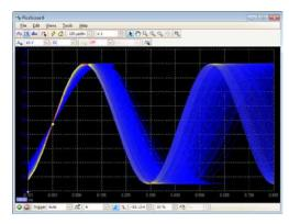
See old and new data superimposed, with new data in a brighter color or shade. This makes it easy to see glitches and dropouts and to estimate their relative frequency. Choose between analog persistence and digital color, or create a custom display mode.
