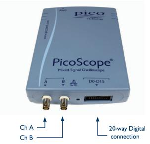
The front panel of the PicoScope 2205 MSO has two BNC analog input channels and a 20-way connection for up to 16 digital signals.
