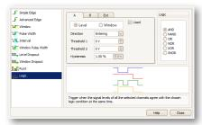
the data you need. All advanced trigger types have adjustable thresholds and hysteresis. The MSOs have a further set of *digital* triggers that can detect any data pattern with optional edge-sensitivity. The *logic* trigger applies the selected Boolean operation to any number of analog, EXT or MSO digital inputs.
