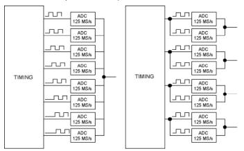
In parallel mode, multiple ADCs are sampled in phase on each channel increasing the resolution to 14 bits (see diagram) at 125 MS/s per channel (70 dB SFDR). If only two channels are required then resolution can be increased to 15 bits, and in single-channel mode all the ADCs are combined to give a 16-bit mode at 62.5 MS/s.
