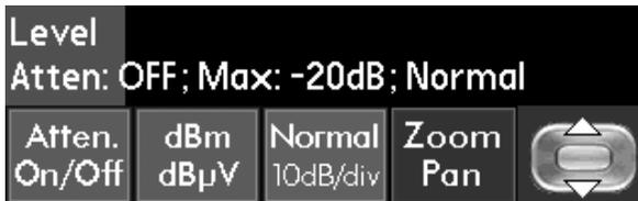
This menu allows the reference level (the level represented by the top of the graticule) to be changed by means of a switchable attenuator. It also allows the display to be vertically zoomed. The current status is shown within the menu area.
