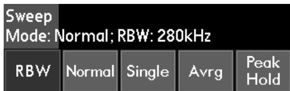
This menu allows the selection of four different sweep modes, and the setting of the resolution bandwidth (RBW). The current sweep mode and RBW are displayed within the menu area.
