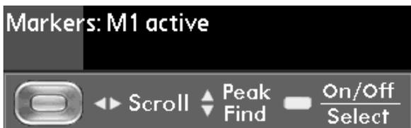
This is not truly a menu as it has no soft keys. Two markers are available shown by yellow and blue vertical lines. The frequency and amplitude at each marker point is displayed below the trace area, along with difference values. The five way navigator is used to control the markers as follows:
