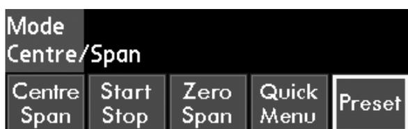
This menu allows the selection of four different modes: Centre/Span, Start/Stop, Zero Span and Quick Menu. The current mode is shown within the menu area. To change mode press the appropriate key after which the unit returns automatically to the home menu.
