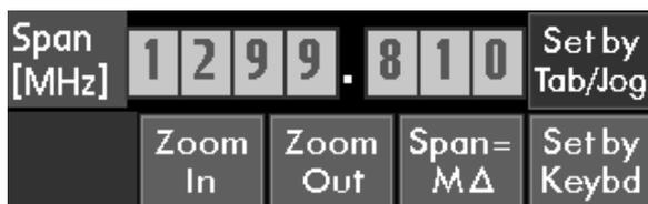
This menu allows the span of the sweep to be set. Values are always in MHz with a maximum resolution of 0.001 (1kHz). The range is 0.320 to 1299.850 MHz or 0.320 to 2699.000 MHz. The current span is displayed within the menu area.
