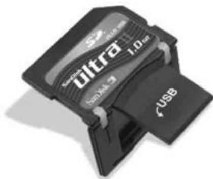
To change the card function to USB, hold the card with the label upwards, and hinge the outer section of the lower half of the card downwards. This exposes a USB connector which can be plugged into a standard USB port on a computer.
