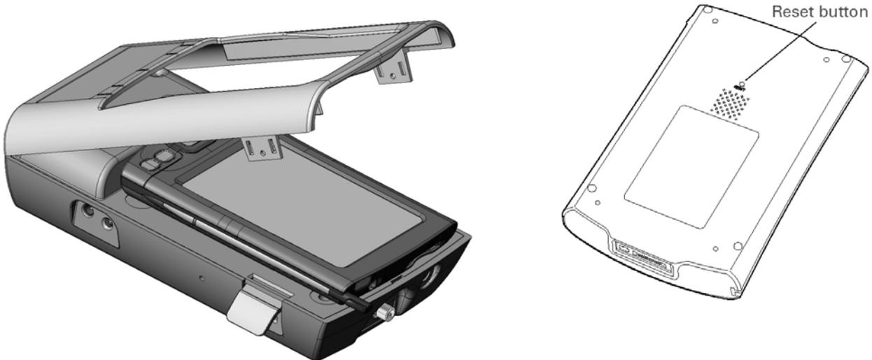
Lift the two latches close to the top of the unit and remove the silver top cover (see drawing). Remove the Palm T|X by gripping its sides and pulling it towards the top edge of the spectrum analyzer. (Note that the connector is a tight fit and that a hard pull may be needed).
